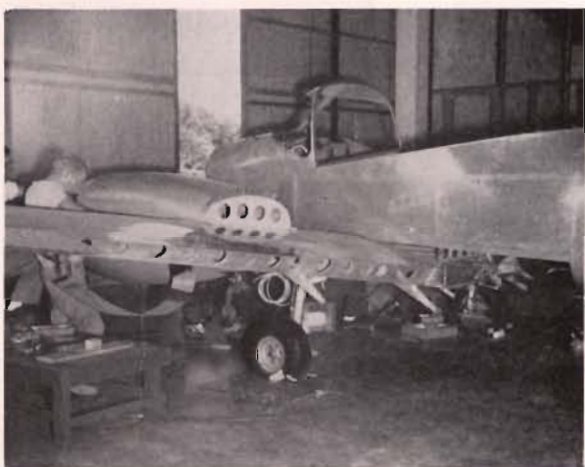
5 After reinforcement, wings are reinstalled and nacelles are added. Engineering and workmanship are equivalent to original.
