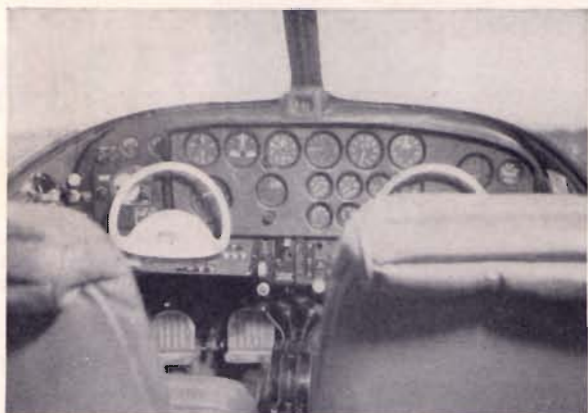
9 New full panel and floor-mounted control pedestal containing throttle, propeller, and mixture controls are fabricated and installed by Riley.
