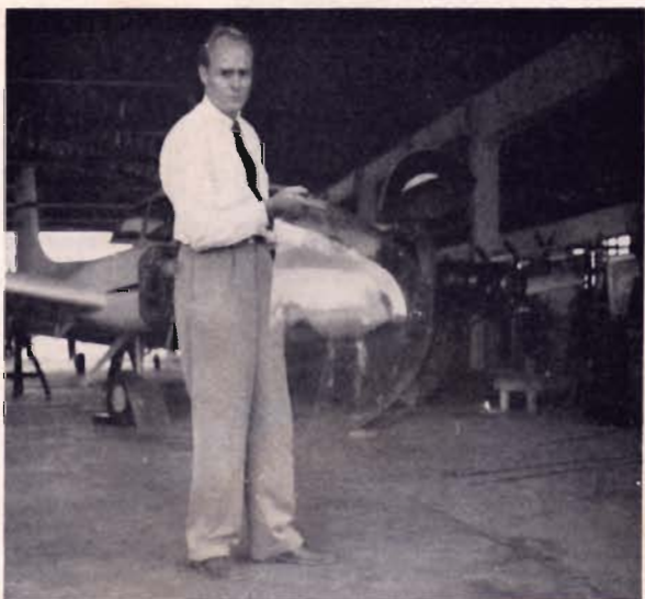
11 New plastic nose piece held here by Frank Peterson, production manager, will replace metal nose section seen in the raised position in the background providing access to the nose compartment. Radio compass loop can then be mounted inside the nose eliminating the drag resulting from external mounting.
