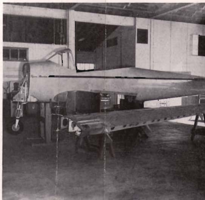
2 First step in conversion is removal of canopy, interior, wings, center section, and tail group.
